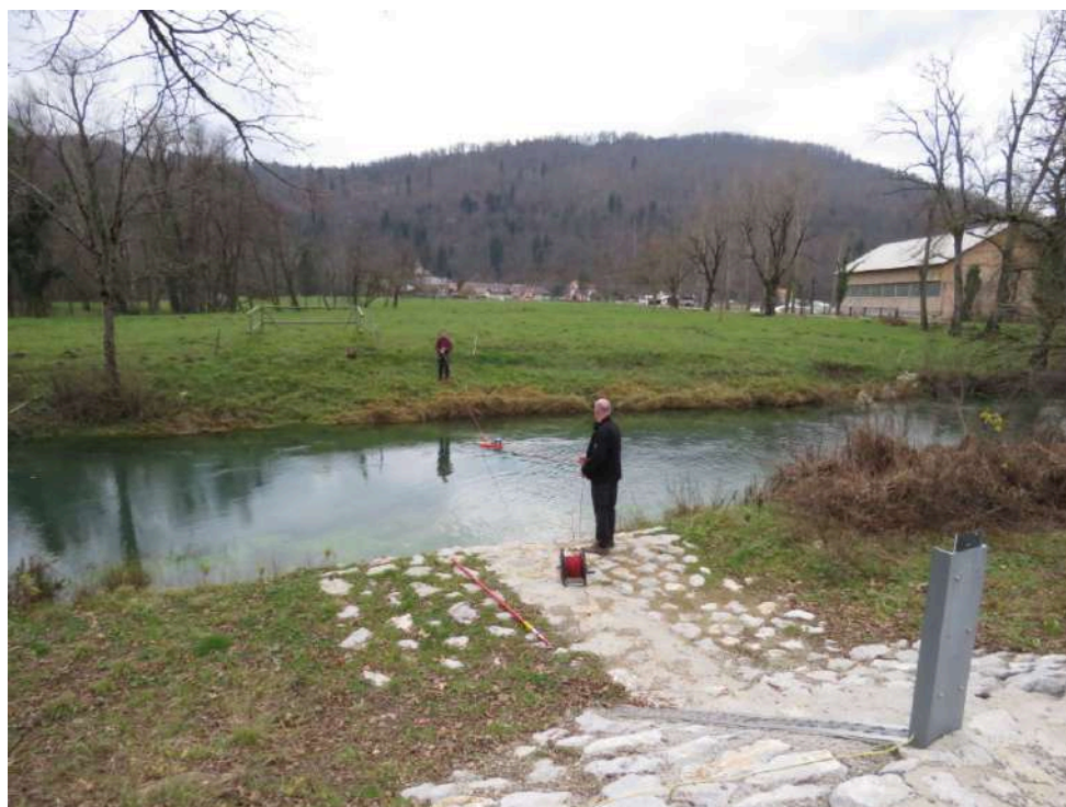
Slika 2. Meritev pretoka izvira Bistre 23. novembra 2017 Figure 2. Discharge measurement of Bistra spring on 23 th of November 2017
