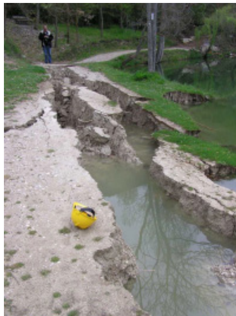
Slika 8. Ob obali jezera Sinizzo so nastale velike in globoke razpoke v tleh (foto: I. Cecić) Figure 8. Big and deep cracks occurred along the shore of lake Sinizzo (Photo: I. Cecić)
