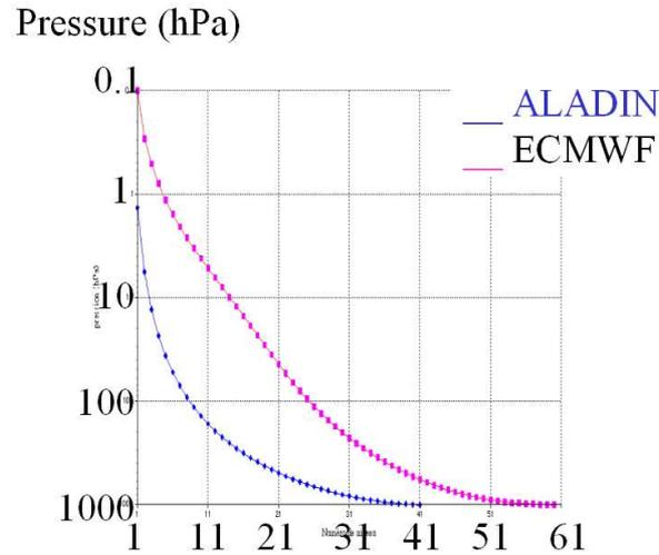
**Figure 2:** Pressure distribution of the vertical levels of the vertical grid of the ALADIN-FRANCE model
