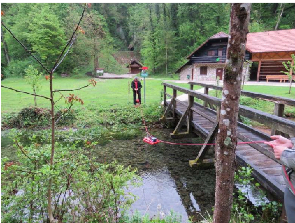
Slika 3. Meritev pretoka na območju izvira Studene v Globočicah 18. aprila 2017 (Foto: arhiv ARSO) Figure 3. Discharge measurement of Studena spring in Globočice on 18 th of April 2017 (Photo: ARSO archive)
