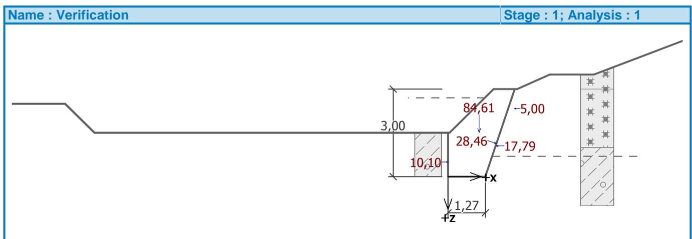
**Bearing capacity of foundation soil****Forces acting at the centre of the footing bottom**
