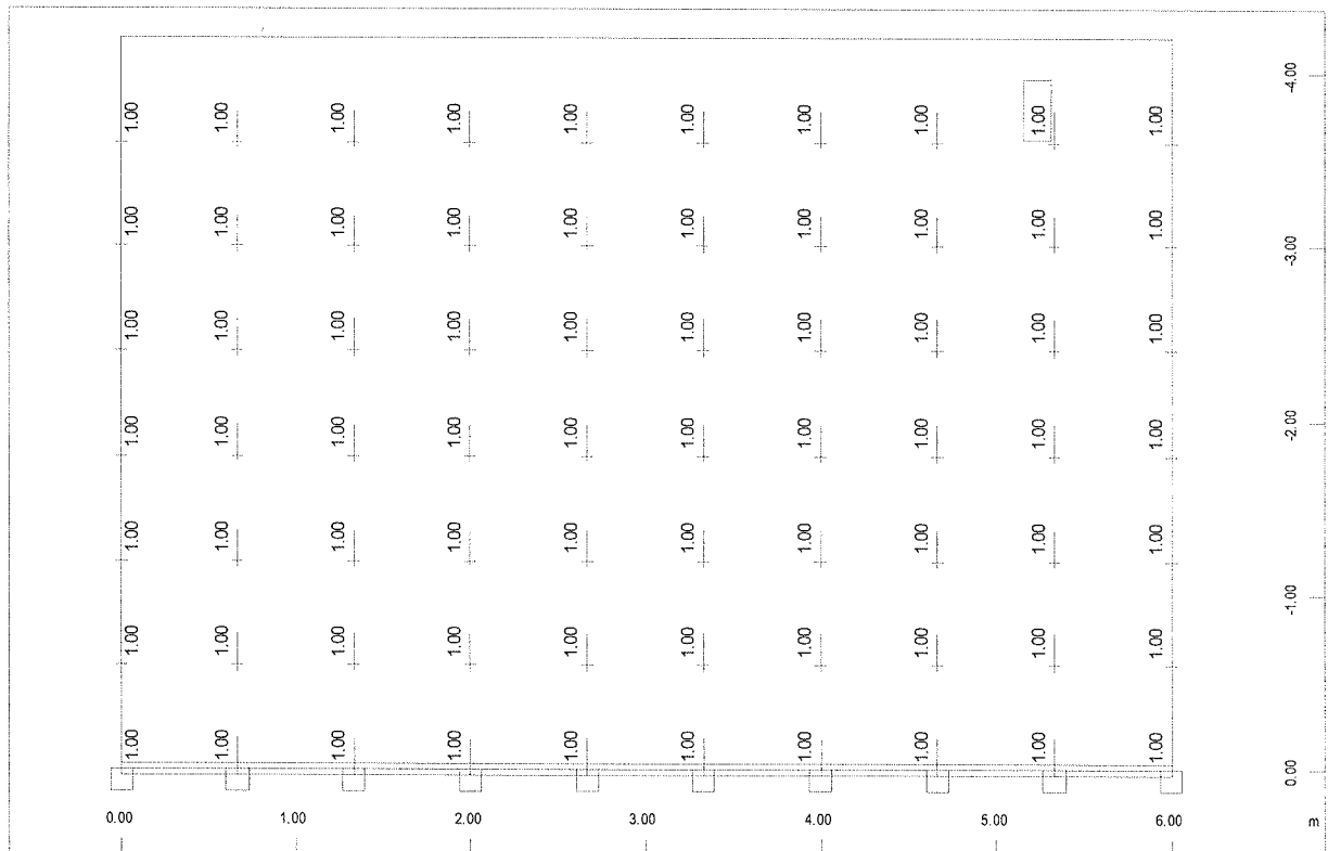
Quadrilateral Elements , lower Principal reinforcements (1st layer) in Node in cm 2 /m, Design Case 2 (Max=1.00)
